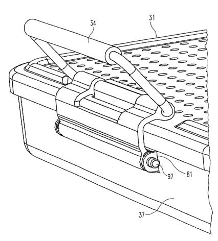
(57) Abstract: A container system for organizing, protecting, sterilizing, storing and delivery of surgical instruments, implants and related devices. An optional cover is removably mounted to a tray and is held thereto by a pair of pivotally mounted handles. Post and button fasteners are removably mounted to the tray and hold rigid and flexible bracketry for securing devices within the assembly.
