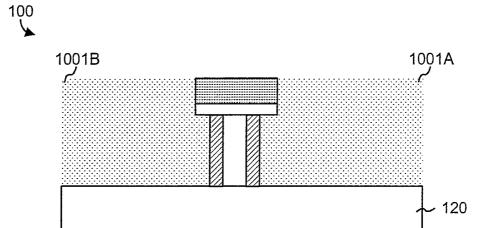
(57) Abstract: A narrow channel FinFET is described herein with a channel width of less than 6 nm. The FinFET may include a fin (140) in which the channel area is trimmed using a  $NH_4OH$  etch or a reactive ion etch (RIE).
