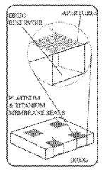
Prior to implanting, drings are sweed in an array of sealend microreservoirs.
