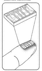
Microchip based implant wirelessly programmed to release drugs inside the body.
