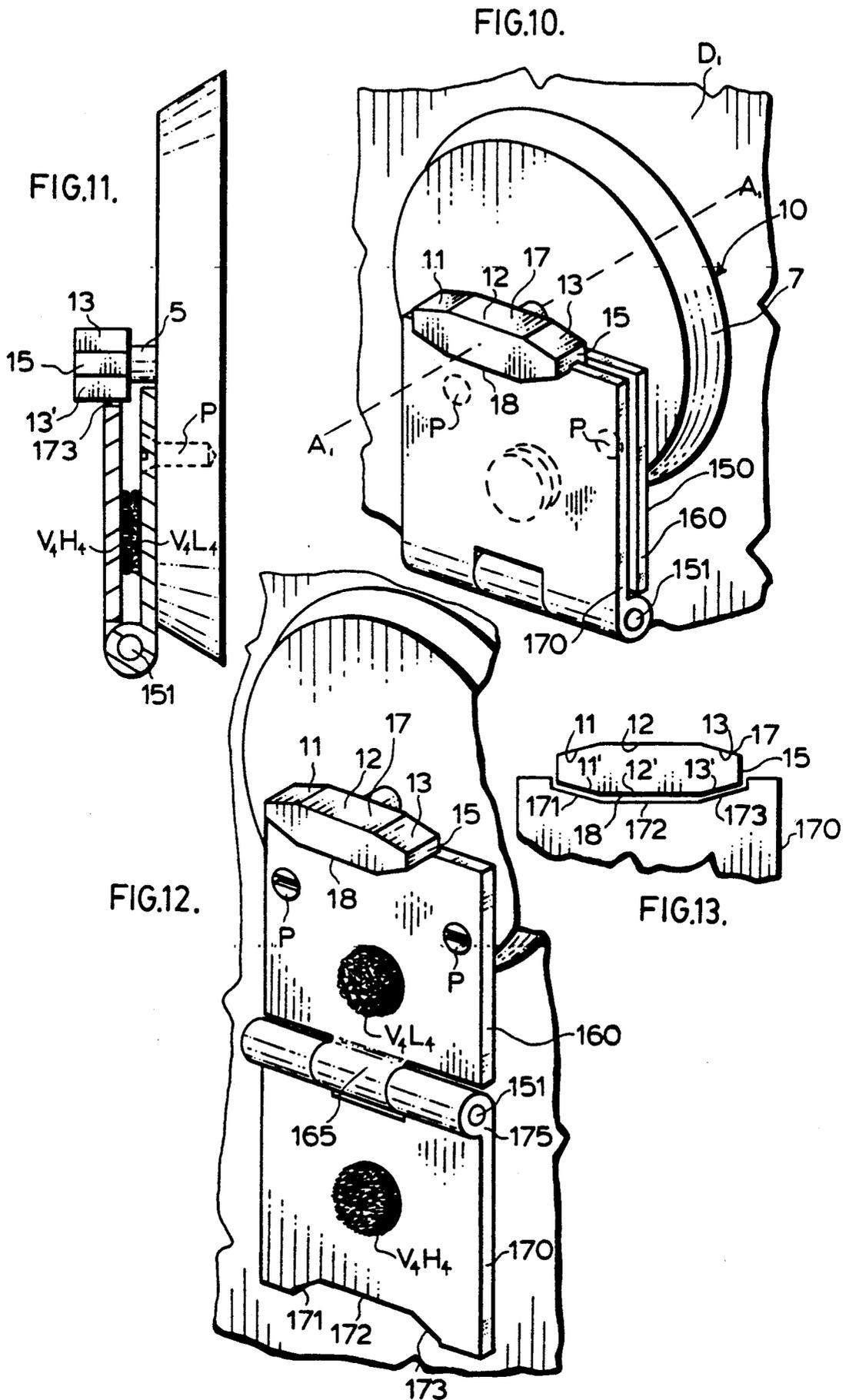
**BLOCKING DEVICE FOR LATCH MECHANISM**
