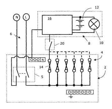
(57) Abstract: A consumer unit (2) is provided comprising at least one current protection device (14). The unit (2) is distinguished in that it further comprises at least one light (8, 10) associated with the unit (2), the at least one light (8, 10) being operatively connected to the at least one protection device (14) whereby the at least one light (8, 10) is energized so as to illuminate the unit (2) when the at least one protection device (14) operates.
