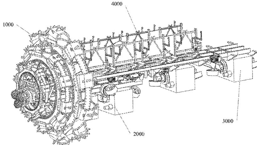
seats. Adjacent ones of the disk drills have the toothed digging buckets facing opposite directions, and the disk drills all rotate in a direction facing a large opening, enabling adjacent two of the three disk drills to rotate in opposite directions. The rotary digging drill further includes three disk drill supports that match the three disk drills in quantity and are configured to support and drive the three disk drills.
