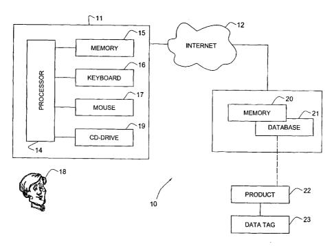
(57) Abstract: A data tag comprising a computer readable medium bearing thereon computer readable program code capable of being run by a computer for automatically presenting to a user data relating to an article of manufacture associated with the data tag.
