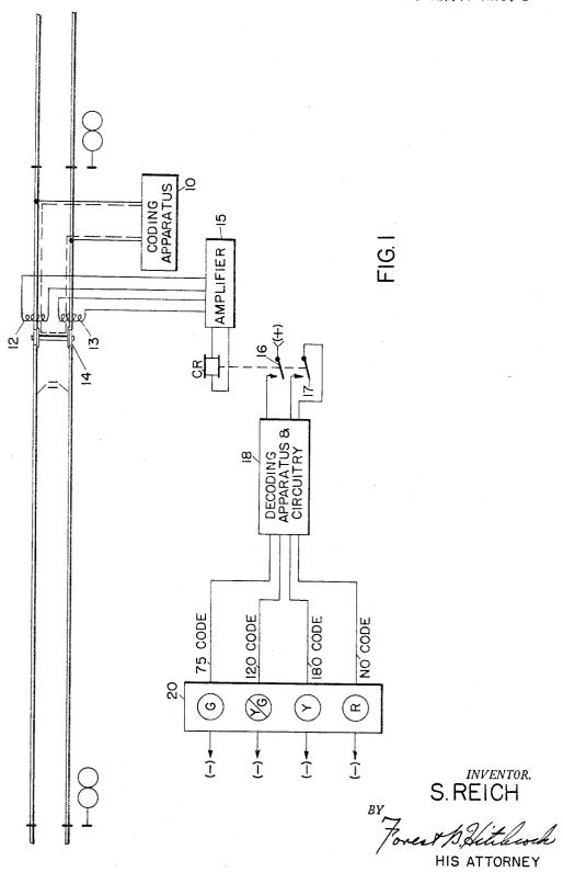
DECODING APPARATUS FOR CONTINUOUS INDUCTIVE TRANSMISSION SYSTEM
