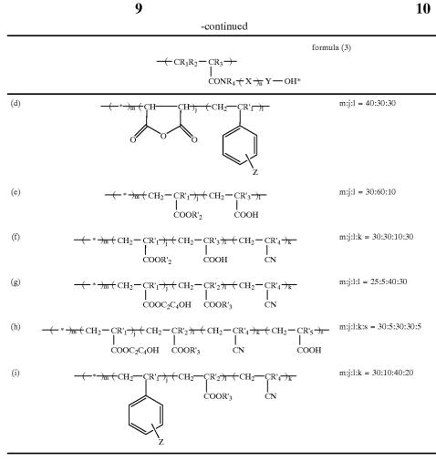
In formula (3), R<sub>1</sub>, R<sub>2</sub>, R<sub>3</sub>, R<sub>4</sub>, X, Y and n are the same  $R_1', R_2', R_3', R_4'$  and  $R_5'$  independently represent a hydrogen atom, an alkyl group or a halogen atom; Z represents an alkyl group, acyloxyalkyl group such as acetoxymethyl or 2-acetoxyethyl, or a halogen atom; and m, j, l, k and s 45 independently represent mol %. Z preferably represents acetoxymethyl.
