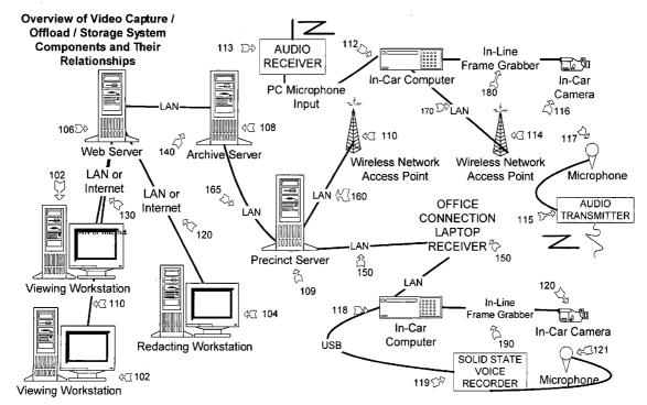
A System for the Capture of Evidentiary Multimedia Data, Live/Delayed Off-Load to Secure Archival Storage and Managed Streaming Distribution
