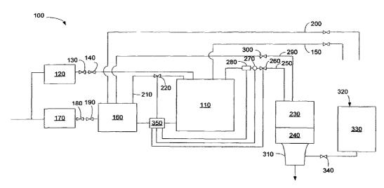
(57) **Abstract:** A method of heating an amount of material positioned within a receptacle. The method may include heating a first volume of water to a predetermined temperature, pressurizing a first volume of steam to a predetermined pressure, releasing the first volume of steam towards the first volume of water so as to force the first volume of water into the receptacle, and heating the material within the receptacle.
