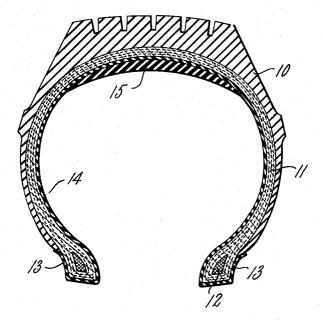
LINER MADE OF BLEND OF BUTYL RUBBER CHEMICALLY MODIFIED BY SULFUR OR ULTRA-ACCELERATOR WITH ANOTHER RUBBER.
