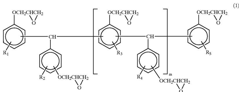
wherein each of  $R_1$  to  $R_5$ , which may be identical or different, is hydrogen atom or an alkyl group having 1 to 5 carbon atoms; and  $m$  is 0 or a positive number of 5 or less, is used as all or a part of the epoxy resin component, from the viewpoint of reducing the bowing by improvement in the glass transition temperature.
