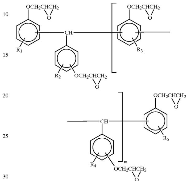
wherein each of R<sub>1</sub> to R<sub>5</sub> is a hydrogen atom and m is 0 or a positive number of 5 or less, wherein said tablet is produced by a process comprising preparing a molten product of said epoxy resin composition in an uncured state and thereafter cooling and solidifying the molten product, and wherein the amount of the tablet that is reduced by heating is less than 0.05% by weight.
