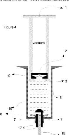
(57) Abstract: A plunger, clip and needle assembly that can be fitted to a conventional syringe barrel thereby allowing the needle assembly to automatically retract after use into a safety compartment located in the plunger, thus preventing re-use of the syringe and needle stick injuries. Retraction of the needle assembly is accomplished from minimal moving parts according to a simple design and requires the user to have no training, the creation of the retracting force is completely intuitive.
