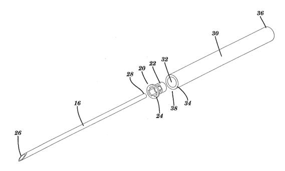
(57) Abstract: A needle-based medical device including a needle guide and a method for constructing the same are disclosed. The needle-based medical device includes a tube having a first lumen; a needle guide which is dimensioned to be inserted into the lumen of the tube, and a needle. The needle is inserted such that an end is positioned in the needle guide. A glue may also be provided to secure the needle guide to the tube. In one embodiment, the tube may be made of extruded plastic.
