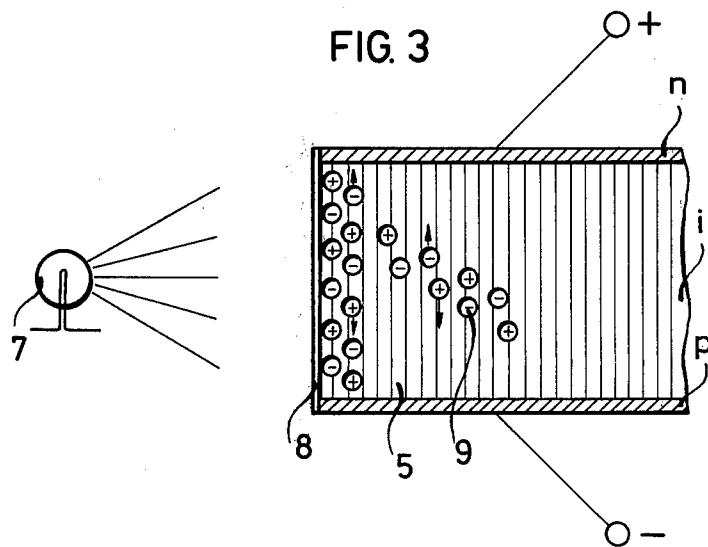
**P-I-N DIODE DETECTOR OF IONIZING RADIATION WITH ELECTRIC FIELD STRAIGHTENING**
