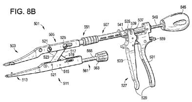
(57) Abstract: An instrument set for an intervertebral expandable spacer having a pair of co-axial annuluses locked together by an engagement member, the set including an inserter/expander having both a rapid expansion mechanism and a fine tuning expansion mechanism.
