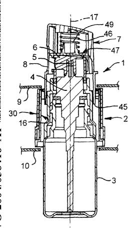
(57) Abstract: This invention relates to a substance dispensing device (1) associated with a usage indicator (2). The device includes a substance storage container (3) and a pump (4) operable to dispense substance from the container (3). The usage indicator includes a movable member (16) that is movable in response to operation of the pump (4). The movable member includes an indication means (29) providing an visual indication of the extent to which substance has been dispensed from the device.
