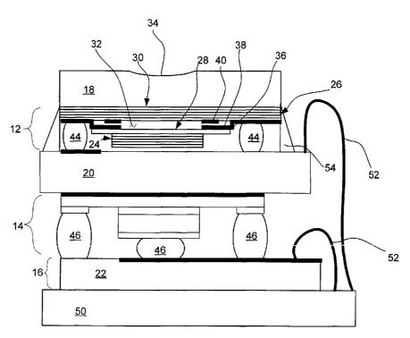
(57) Abstract: A spectrally tunable optical detector and methods of manufacture therefore are provided. In one illustrative embodiment, the tunable optical detector includes a tunable bandpass filter, a detector and readout electronics, each supported by a different substrate. The substrates are secured relative to one another to form the spectrally tunable optical detector.
