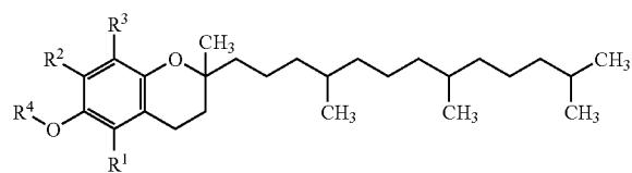
[0034] where  $R^1$  is hydrogen or methyl,  $R^2$  is hydrogen or methyl,  $R^3$  is hydrogen or methyl, and  $R^4$  is hydrogen or an acyl radical having from 1 to 20 carbon atoms.
