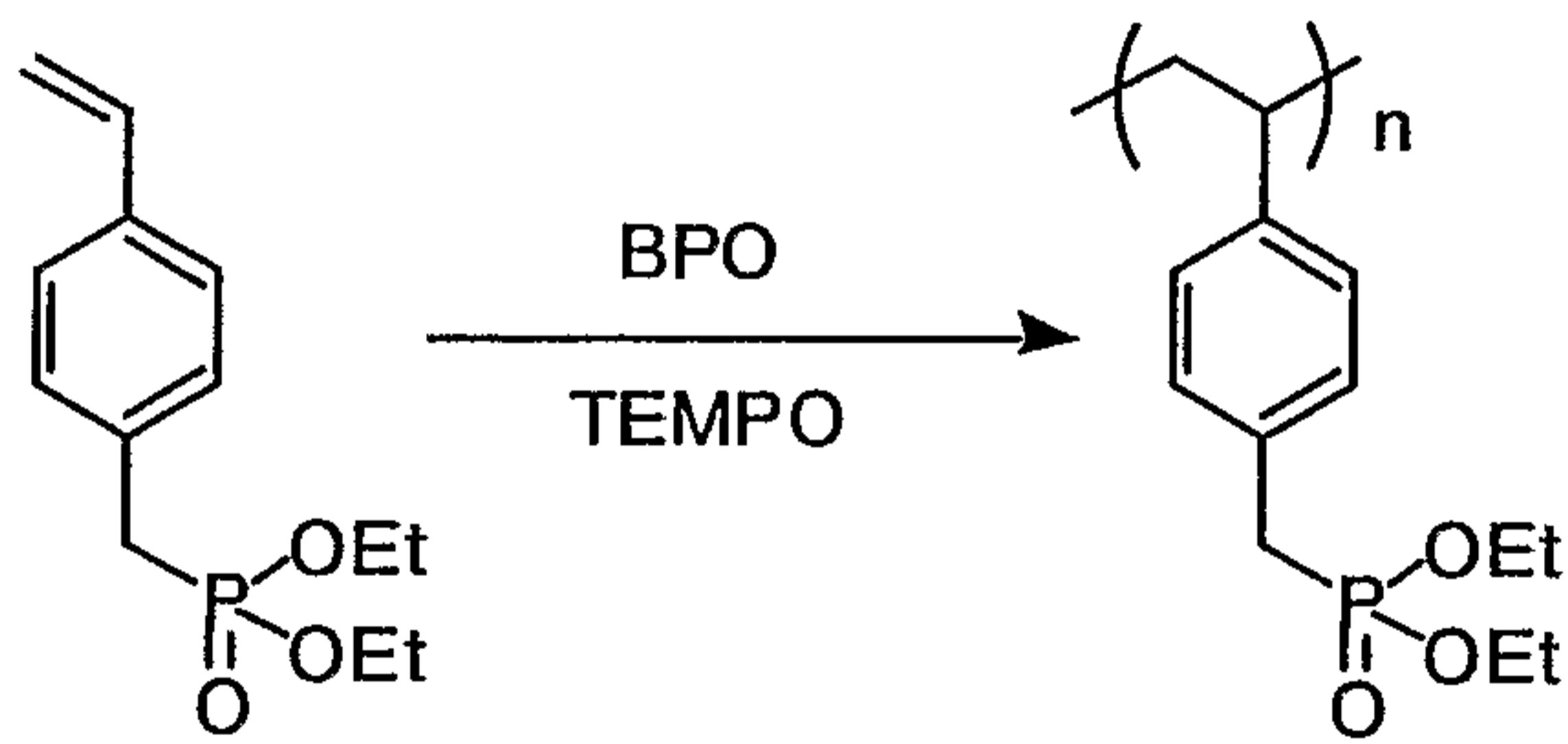
5.0 g (20 mmol) of diethyl 4-vinylbenzylphosphonate, 48 mg (0.20 mmol) of benzoyl peroxide (BPO) and 41 mg (0.26 mmol) of 2,2,6,6-tetramethyl-1-piperidinyloxy (TEMPO) were placed in a 50-mL eggplant-shaped flask with three way cocks, for deaeration by freeze-thaw cycle. Subsequently, the inside of the flask was substituted with argon. The reactor was placed
