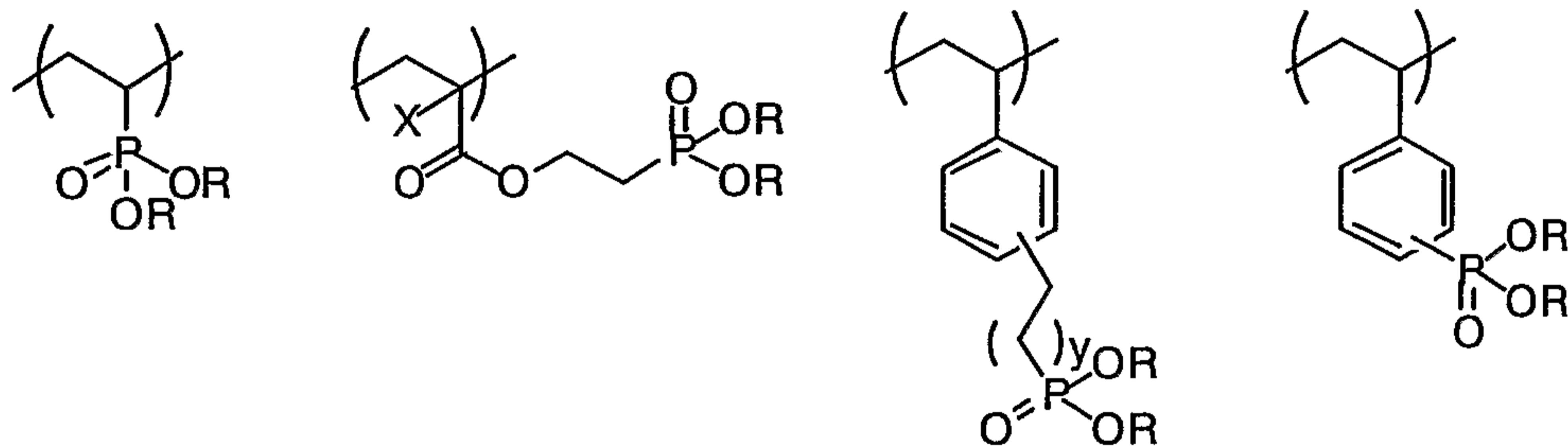
Additionally, R in the formula (4) independently represents hydrocarbon, an aromatic ring, hydrogen, a metal ion or onium ion and individual Rs may be the same or different. In terms of ready synthesis, the Rs are preferably the same. Examples of R as the hydrocarbon include chain-like hydrocarbons with one or more to 18 or less carbon atoms, which
