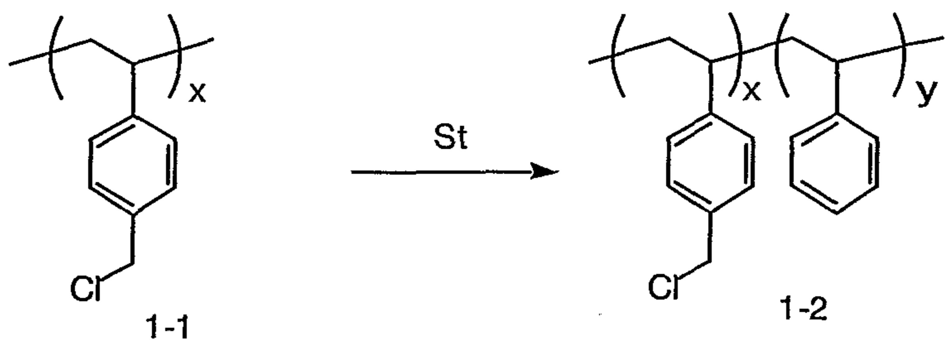
10 g (96 mmol) of styrene (St) and 3.0 g of poly(4-chloromethylstyrene) (1-1) were placed in a 50-mL eggplant-shaped flask with three way cocks, for deaeration by freeze-thaw cycle. Subsequently, the inside of the flask was substituted with argon. The reactor was placed in an oil bath at 125°C, for agitation for 25 hours. The reaction solution was cooled to ambient temperature and was diluted with THF,
