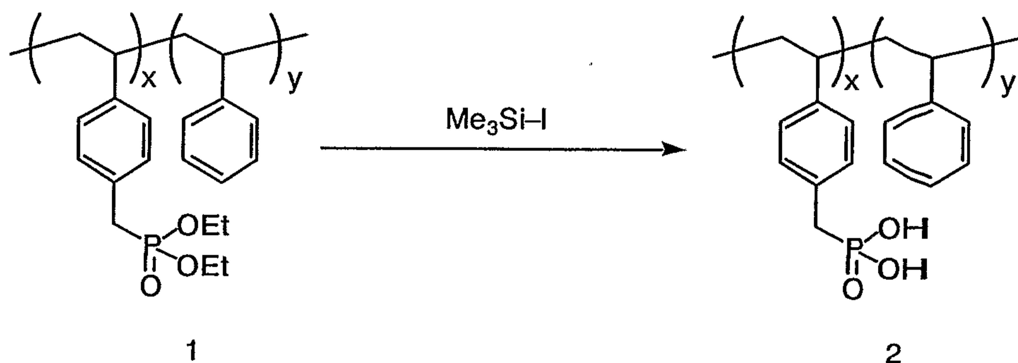
A solution of the listed compound No. 1 in anhydrous dichloromethane was placed in an eggplant-shaped flask with two necks in Ar atmosphere, to which iodotrimethylsilane was added to the solution while the solution was cooled in an ice bath. The reaction solution was back to ambient temperature, for agitation for 24 hours as it was. An aqueous saturated solution of sodium sulfite was added to the reaction solution, for agitation, until the reaction solution was colorless.
