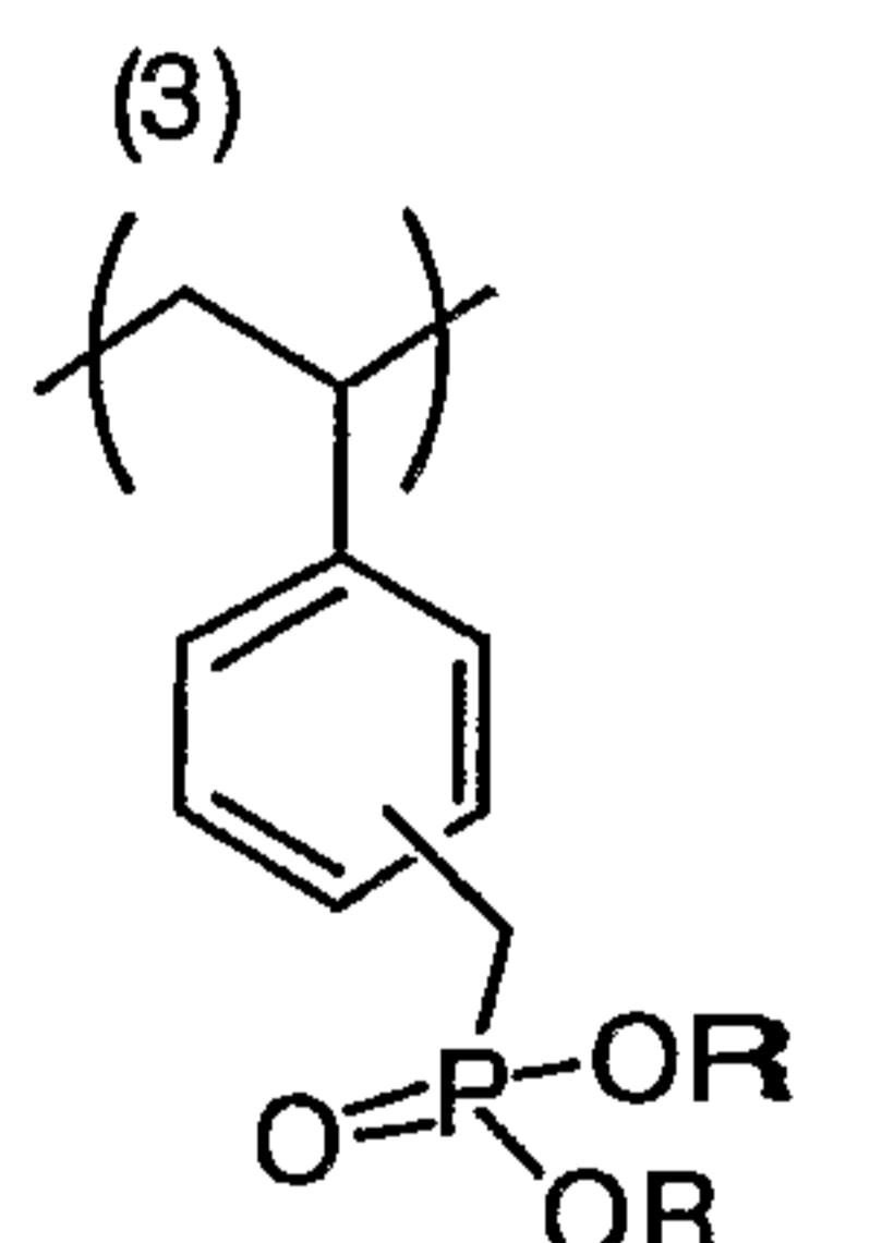
where R independently represents hydrocarbon, an aromatic ring, hydrogen, a metal ion or onium ion.
