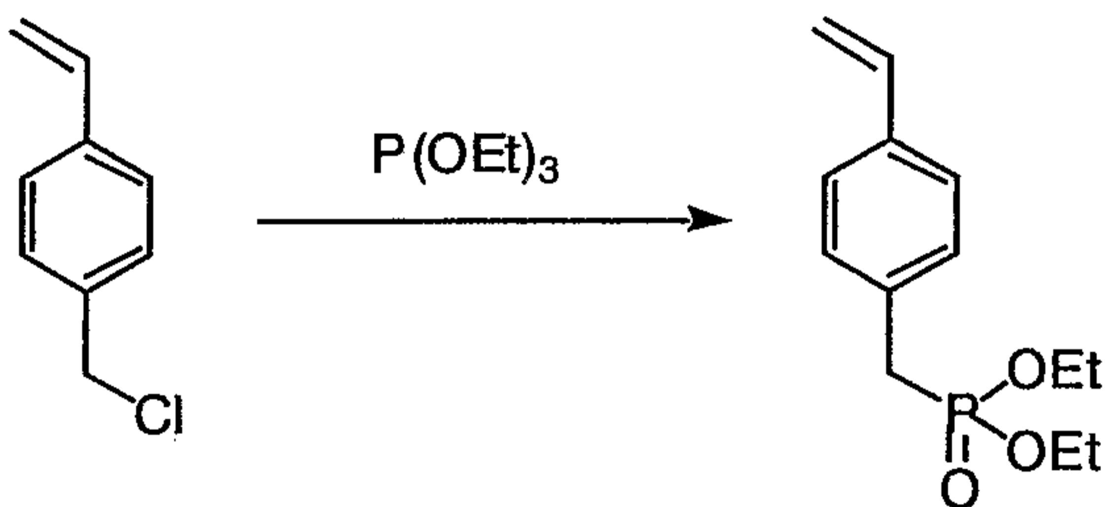
15 g (90 mmol) of triethyl phosphite, 11 g (75 mmol) of 4-chloromethylstyrene and hydroquinone (100 mg) were placed in a 50-mL eggplant-shaped flask with three necks, for agitation at 100°C for 44 hours. The reaction solution was back to ambient temperature, from which unreactive triethyl phosphite and CMS were distilled off under reduced pressure. The product was purified by silica gel column chromatography
