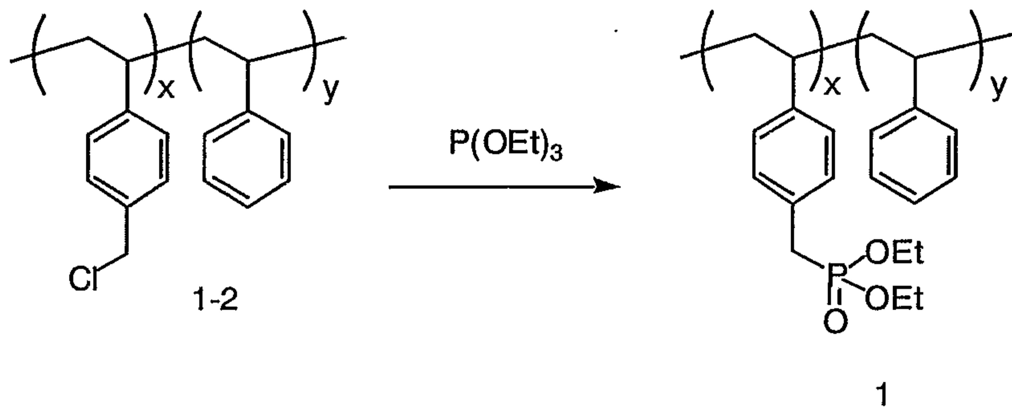
20 g (120 mmol) of triethyl phosphite and 8.0 g of poly(4-chloromethylstyrene)-b-polystyrene (1-2) were placed
