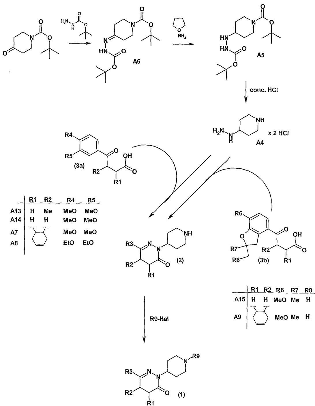
Reaction scheme 1 shows that the compounds of formula 1 can be, for example, prepared starting from 4-oxo-piperidine-1-carboxylic acid tert-butyl ester which is reacted in a first reaction step with tert-butylcarbazate to give 4-(tert-Butoxycarbonyl-hydrazono)-piperidine-1-carboxylic acid tert-butyl ester (starting compound A6). Compound A6 is reduced with, for example, the boran tetrahydrofuranate com-
