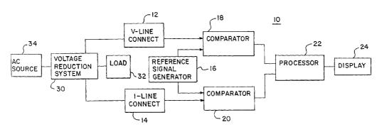
(57) Abstract: A method and system for measuring an amount of power reduction is provided. A percentage or absolute reduction from full power is calculated. The percentage or absolute reduction in power is determined from voltage and current duty cycle information extracted from a comparison of the source waveform to a reference waveform.
