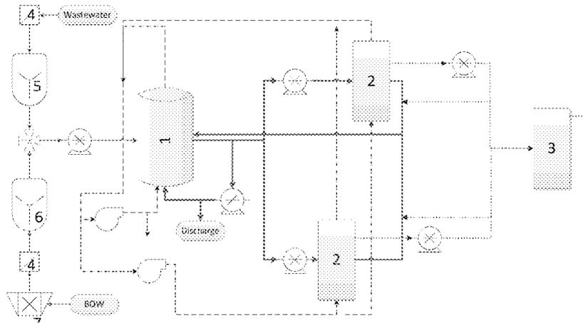
continuously feeding at least one anaerobic reactor, with previously sieved wastewater and feeding biodegradable organic waste—BOW—also previously sieved, said reactor being coupled to at least one gasified filtration membrane, with recirculation of biogas from the reactor,
