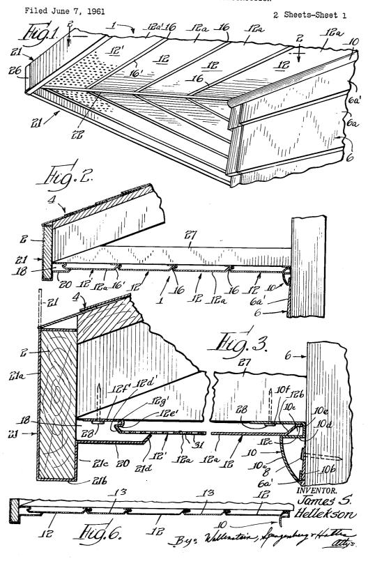
PREFABRICATED SOFFIT CONSTRUCTION
