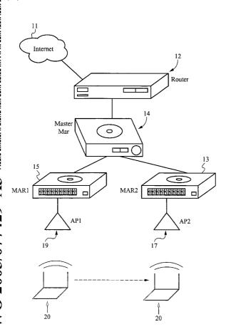
(57) Abstract: Method and apparatus (Fig. 3) for allowing mobiles (20) to roam between subnets using access points (17, 19), and a router (12) connected to the Internet (11).
