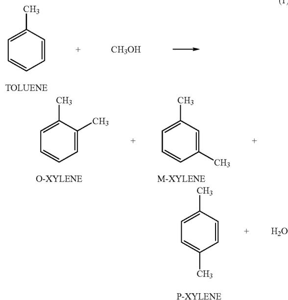
Thermodynamic equilibrium compositions of o-, m-, and p-xylenes may be around 25, 50 and 25 mole %, respectively, at a reaction temperature of about 500° C. Such toluene methylation may occur over a wide range of temperatures, however. Para-xylene can be separated from mixed xylenes by a cycle of adsorption and isomerization. Byproducts such as C9+ and other aromatic products can be produced by secondary alkylation of the xylene product.
