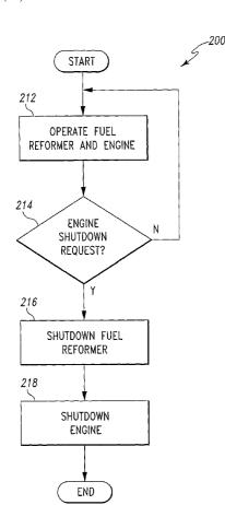
(57) Abstract: A method of operating a power system (10) including a fuel reformer (11) and an internal combustion engine (12) is disclosed. The engine is shutdown subsequent to shutdown of the fuel reformer (11). A fuel reformer system for supplying a reformate gas to the engine is also disclosed.
