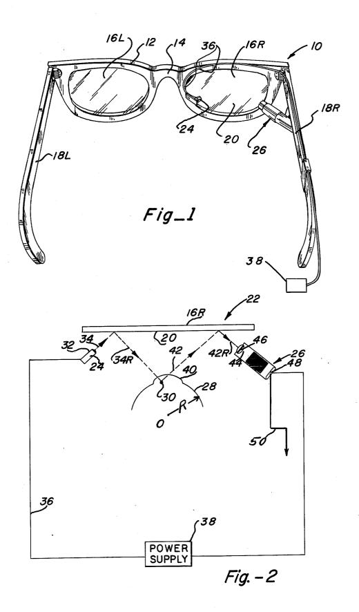
METHOD AND APPARATUS FOR MONITORING THE POSITION OF THE EYE
