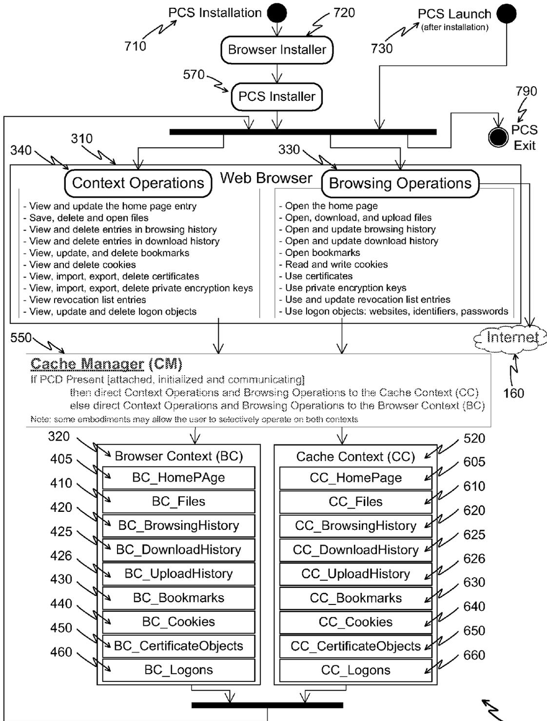
Figure 7 Portable Caching System Activity Diagram
