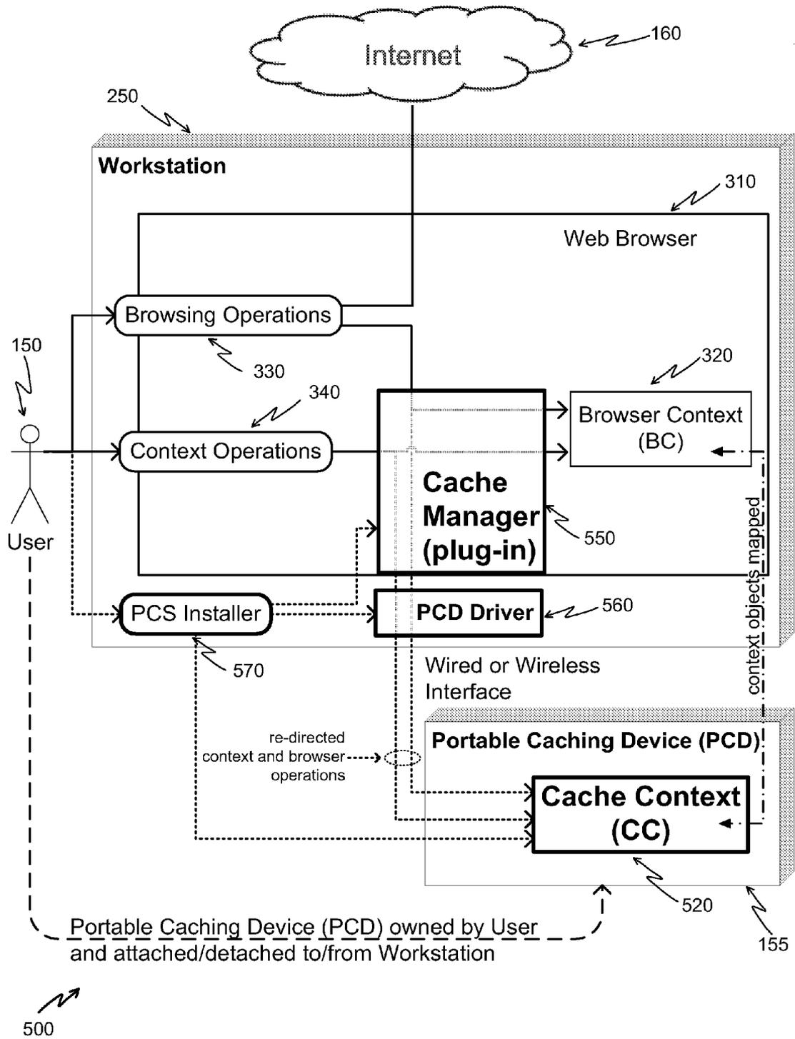
Figure 5 Portable Caching System Identifying Inventive Subject Matter
