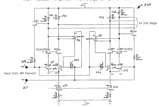
Main Reader Amplifier First Stage Simplified Schematic
