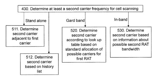
nication device then performs (440) cell scanning on the determined at least second carrier frequency.
