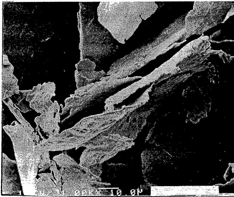
FIG. 1 Conventional Tantalum Flake 1000X Magnification
