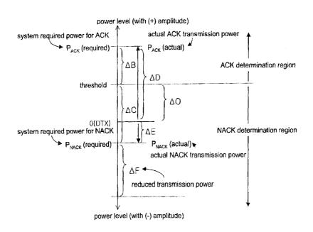
NACK determination region ACK determination region actual NACK transmission power actual ACK transmission power power level (with (+) amplitude) P<sub>ACK</sub> (actual) P<sub>ACK</sub> (actual) BACKGROUND ART power level (with (-) amplitude) ΔΑ ΔΑ Eg. 0(DTX) system required power for NACK ► P<sub>NACK</sub> (required) → P<sub>ACK</sub> (required) threshold system required power for ACK
