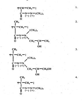
The polyvinyl aminimides of the present invention are known to the art. Aminimides suitable for use in the present invention are prepared by reacting a hydrazine with the appropriate vinyl acid chloride. Polymerization may be achieved by free radical polymerization 5 techniques. Additional details regarding preparation of the monomers and formation of the polymers may be found in U. S. Pat. No. 3,641,145, issued Feb. 8, 1972, incorporated by reference herein in its entirety
