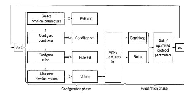
End Set of optimized parameters protocol Preparation phase Conditions Rules Apply the values to: Condition set PAR set Rule set Values Configuration phase physical parameters physical values Configure Measure conditions Configure Select rules Start
