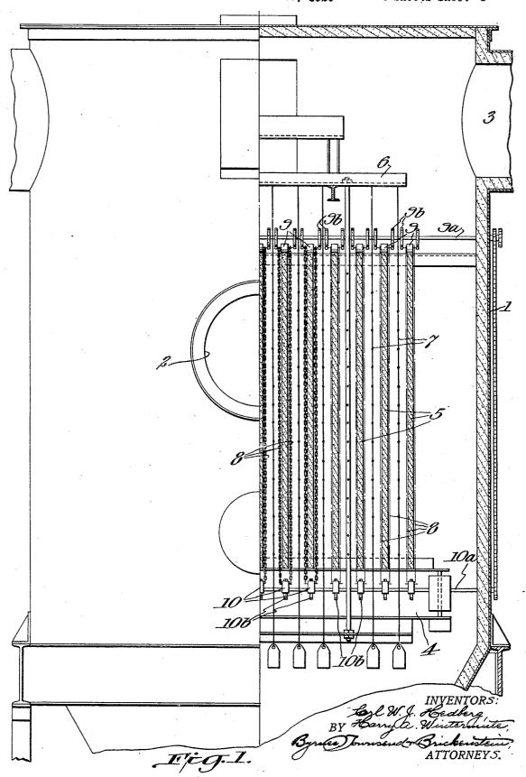
PRECIPITATOR CLEANING DEVICE
