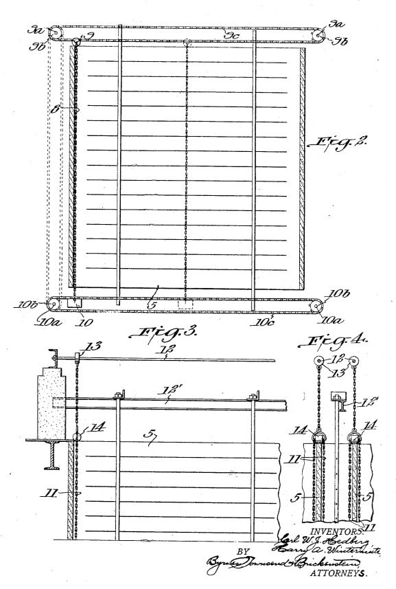
PRECIPITATOR CLEANING DEVICE
