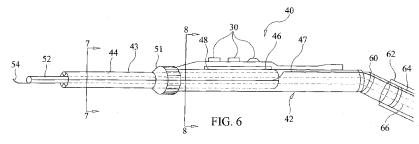
(57) Abstract: A surgical pencil that enables simultaneous cutting with an electrode and coagulating with a coagulating material while also performing smoke evacuation. Several different sources of energy can be used for both open procedures and laparoscopy including electrosurgery and argon beam coagulation. In argon beam coagulation (ABC), current is applied to tissue by a directed beam of ionized argon gas which causes a uniform and shallow coagulation surface thereby stopping blood loss.
