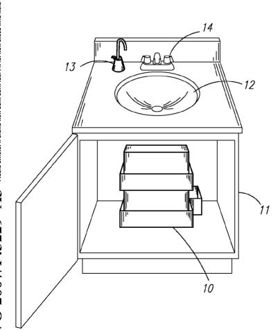
(57) Abstract: A bladder tank for storing a liquid includes an outer housing and an inner bladder. A storage platform is mounted to the outer housing for storing an article thereon. Miscellaneous articles can be stored on the storage platform. The bladder tank can be mounted in a cabinet beneath a sink.
