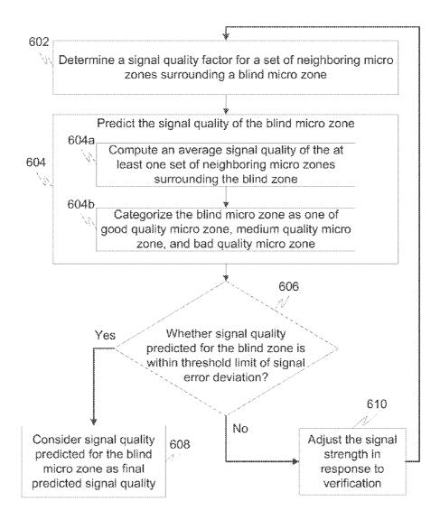
FIG. 6: Methods And Systems For Determining Radio Coverage In Wireless Communication Networks
