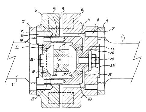
(57) Abstract: A flexible shaft coupling is provided with a ball joint (12, 13) in the form of two spherical bearings which are so arranged that their bearing faces each form a part of a spherical surface whose centre is centrally positioned between the two coupling halves (5, 6) of the shaft coupling.
