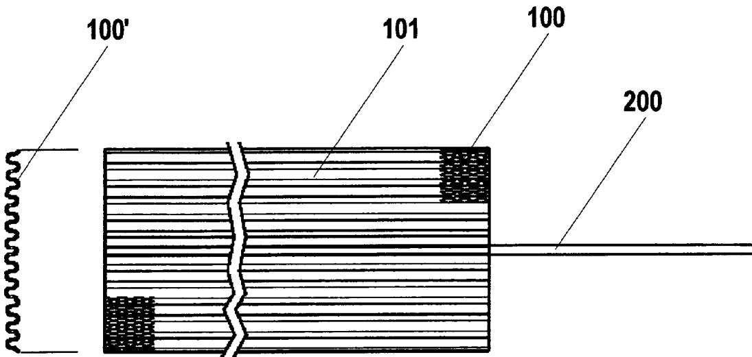
(57) Abstract: It is described a cathodic protection system of reinforced concrete structures with discrete anodes obtained starting from a corrugated planar substrate welded to a longitudinal current collector. The anodes of the invention are particularly suitable for being installed rolled in cylinders, with their axis parallel to the current collectors, positioned inside holes made in the concrete of the structure to be protected.
