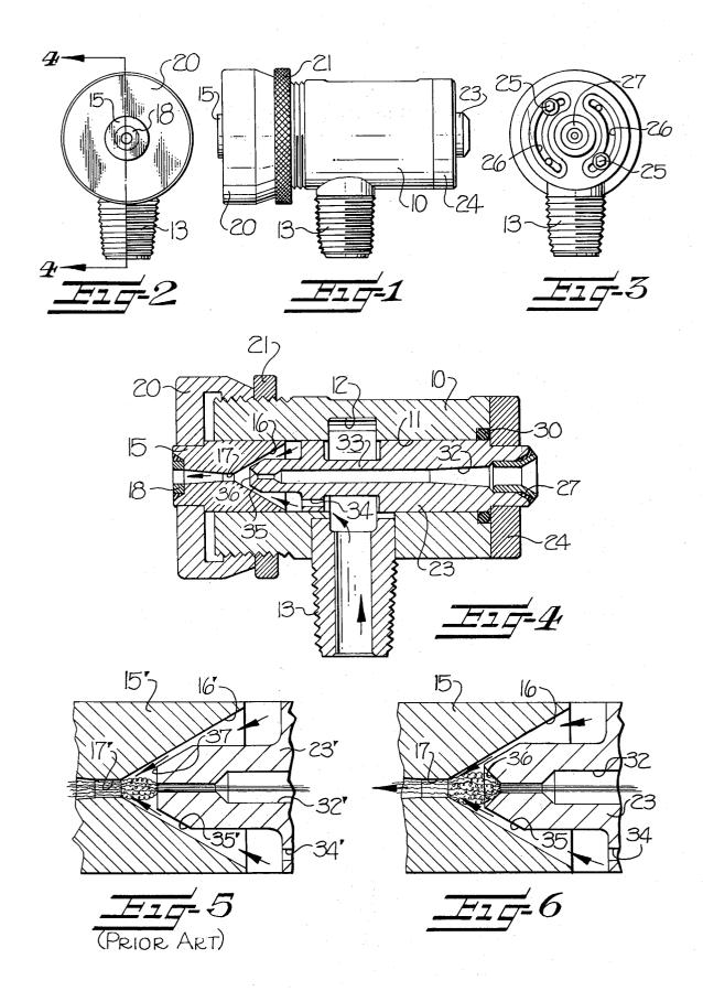
This invention relates generally to a yarn texturing air jet and more particularly to an improvement in the turbulence chamber of the air jet to enhance the crimps, 5 curls and loops produced in the filaments of the yarn and to permit a faster and more economical operation.
