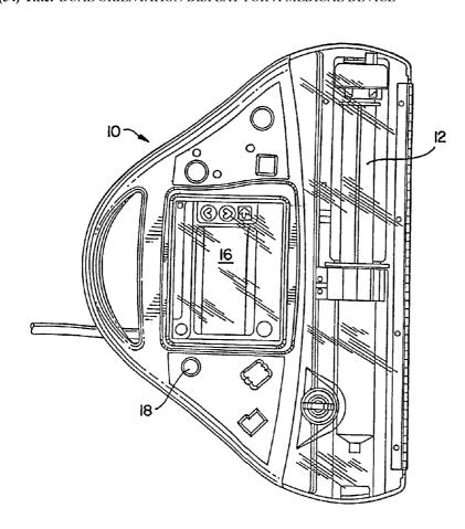
(57) Abstract: medical device(10) is disclosed. The device (10) is adaptable for configuration in various positions. In the preferred embodiment, the device (10) comprises an infusion pump (12) for dispensing a medical fluid to a patient. A controller (14) is operably connected to a display (16) and the pump (12). display (16) is operably responsive to the position of the pump (10) wherein information on the display (16) can be easily viewed.
