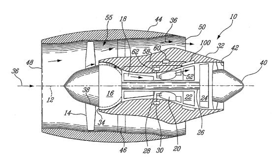
(57) Abstract: An apparatus and method for selectively cooling a gas turbine engine component for the purpose of controlling blade tip clearance during transient conditions, wherein cooling air is admitted intermittently according to a desired a duty cycle based on a present or anticipated transient condition.
