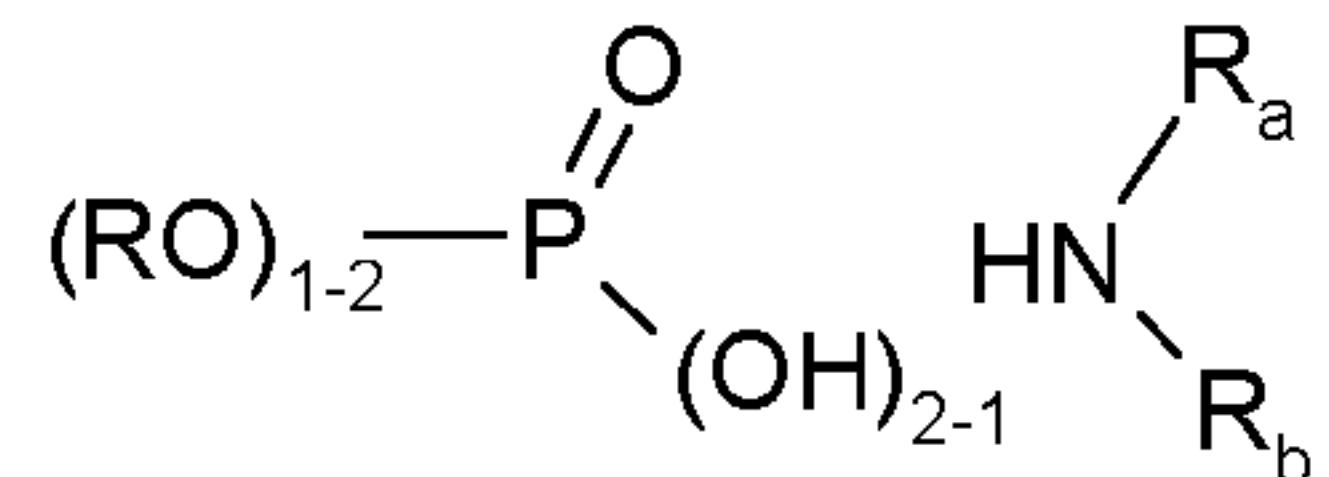
Wherein R represents  $C_3$ - $C_{18}$ alkyl and  $R_a$  and  $R_b$  represent  $C_6$ - $C_{20}$ alkyl, such as products named as amines, C11-14-branched alkyl, monohexyl and dihexyl phosphates.
