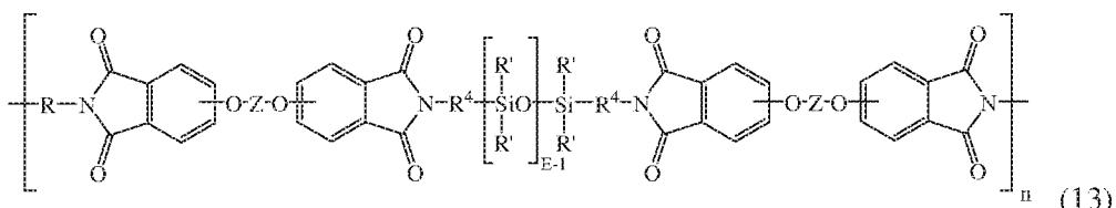
wherein R' and E of the siloxane are as in formula (9), the R and Z of the imide are as in formula (5), R<sup>4</sup> is the same as R<sup>4</sup> as in formula (12), and n is an integer from 5 to 100. In a specific embodiment, the R of the etherimide is a phenylene, Z is a residue of bisphenol A, R<sup>4</sup> is n-propylene, E is 2 to 50, 5, to 30, or 10 to 40, n is 5 to 100, and each R' of the siloxane is methyl.
