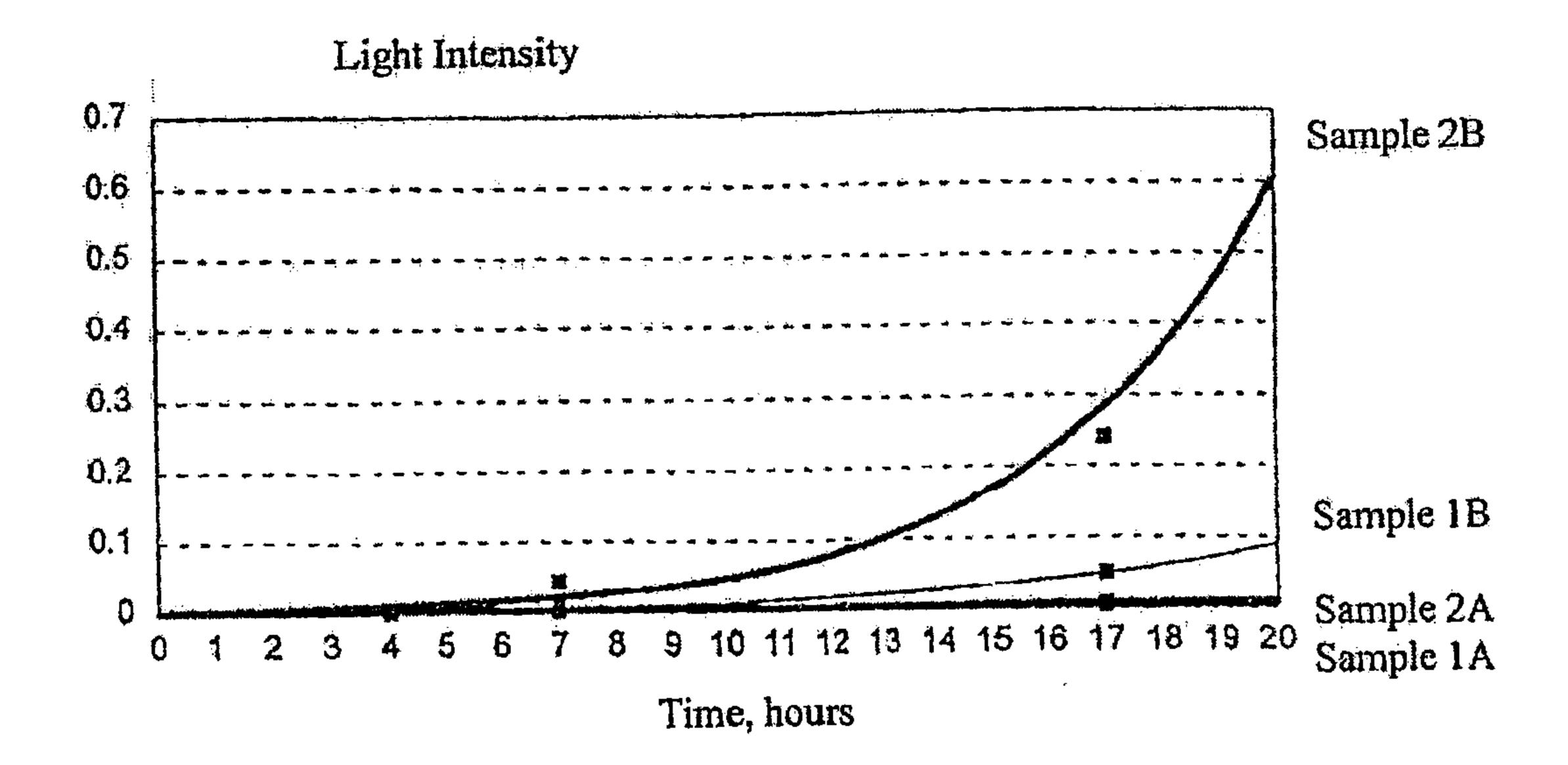
Figure 1 illustrates the light intensity, as measured by BioOrbit luminometer 1253, as a function of incubation time following centrifugation of slurries according to Example 3.
