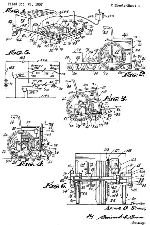
DRIVING AND STEERING APPARATUS FOR WHEEL CHAIRS
