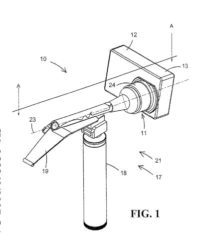
(57) Abstract: Adaptor for mounting a handheld portable consumer device having a built-in digital camera (12) and a display screen on a handheld portable laryngoscope (17) having an optical system (13) for "viewing a subject's laryngeal region during endotracheal intubation for rendering a handheld portable medical viewing assebly for displaying medical images of subject laryngeal region during endotracheal intubation.
